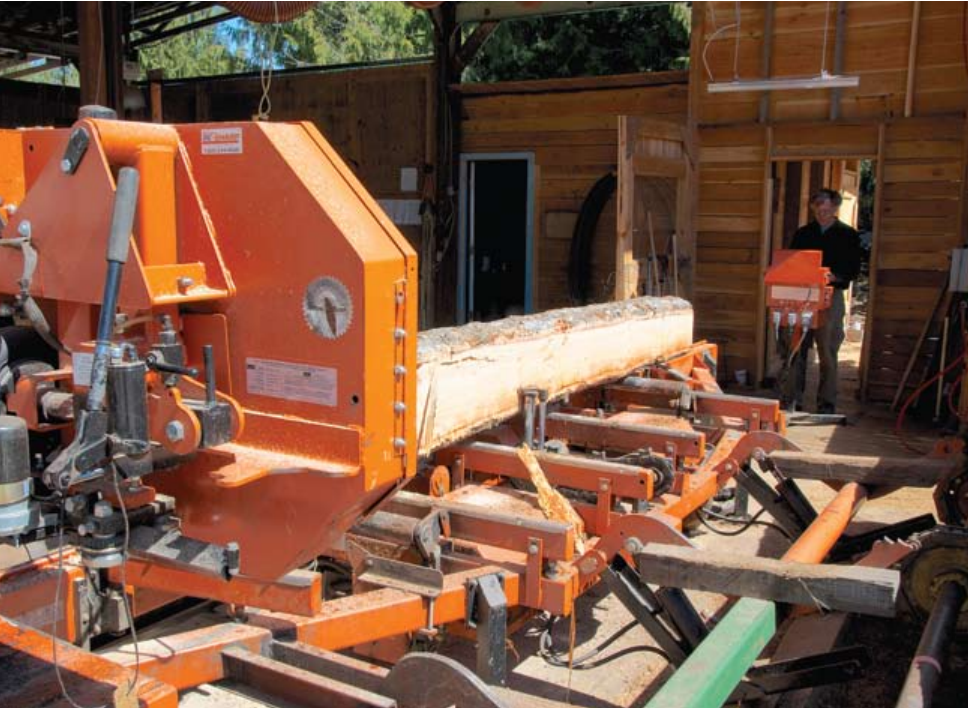
The Harrop - Procter Forest Products sawmill in action. A Douglas fir log is being milled into a timber for a timber frame home by David Strom of Harrop - Procter Forest Products. Photo courtesy of Ursula Heller
