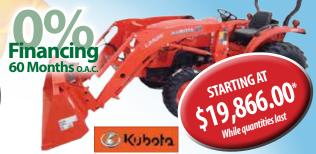
L-series standard 25hp (non DPF) tractor that's powerful enough to tackle a wide range of tasks, yet nimble enough to provide the precision performance and ease of use that you need. With a HST transmission that offers simple forward and reverse change for optimal operating and ease of front end loader work. Strong 1918lb 3pth lift capacity and power steering make operating this tractor a dream.
