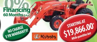
L-series standard 25hp (non DPF) tractor that's powerful enough to tackle a wide range of tasks, yet nimble enough to provide the precision performance and ease of use that you need. With a HST transmission that offers simple forward and reverse change for optimal operating and ease of front end loader work. Strong 1918lb 3pth lift capacity and power steering make operating this tractor a dream.
